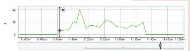
Graph indicates high and variable overall acceleration, an indication of potential cavitation.
