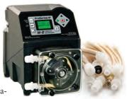
trol systems design, which permits connection to SCADA systems and other remote controllers, for chemical dosing control via either a 4-20mA signal, a high-speed digital pulse input, or a slow pulse for batching type applications. The head roller assembly has two CNC-machined squeeze rollers and two alignment rollers. The firmware is field upgradable. Output is from .007 to 15 gph with output pressure ratings to 125 psi. It is certified NEMA 4X, IP66, NSF STD 61, CE, and ETL.
