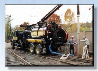
**SEWER & CATCH BASIN CLEANING** Single and double-pump jet-vac combination units with line jetting capabilities of 175 gpm. Catch basin cleaning available with per hour or per basin pricing.
