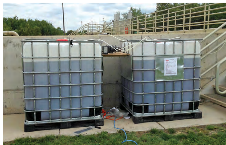
The pilot study setup includes two bulk chemical tanks for polyaluminum chloride. Peristaltic pumps and tubing enable discharge of the chemical over the basin walls and on top of the outfall weirs.
