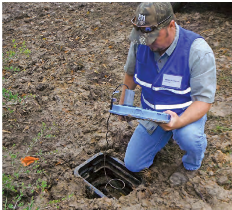
Ultrasonic meters measure flow using sound waves at frequencies above the range of human hearing. The sound waves are generated by applying a small voltage to a piezoelectric transducer in the meter.
