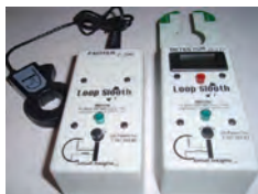
Loop Slooth Exciter/Detector ground loop diagnostic device from Circuit Insights
