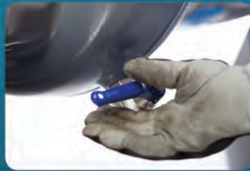
Drainage port for quick and clean servicing
