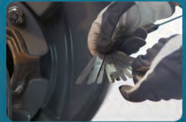
Simplified impeller check and adjustment with roll back cart and telescopic inlet
