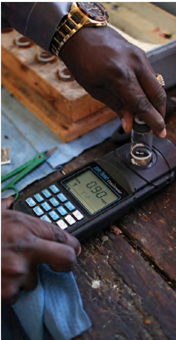
A portable colorimeter (Hach) is used to test a water sample.
