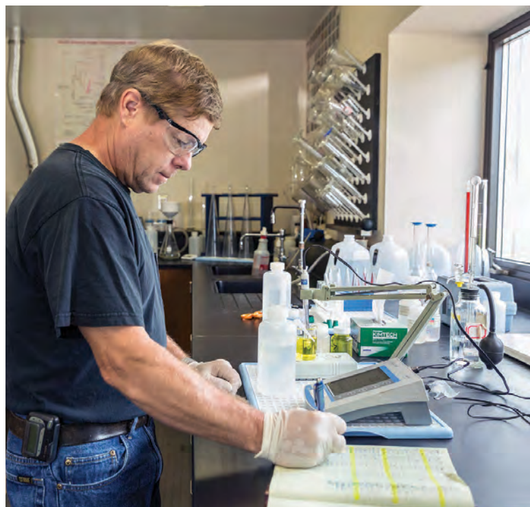
Operator Howard Kimball runs a check on an Accumet pH meter (Cole-Parmer).
