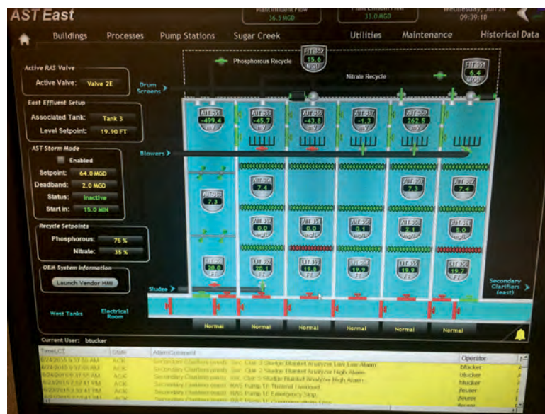
The sensor network integrates with the facility's SCADA system.
