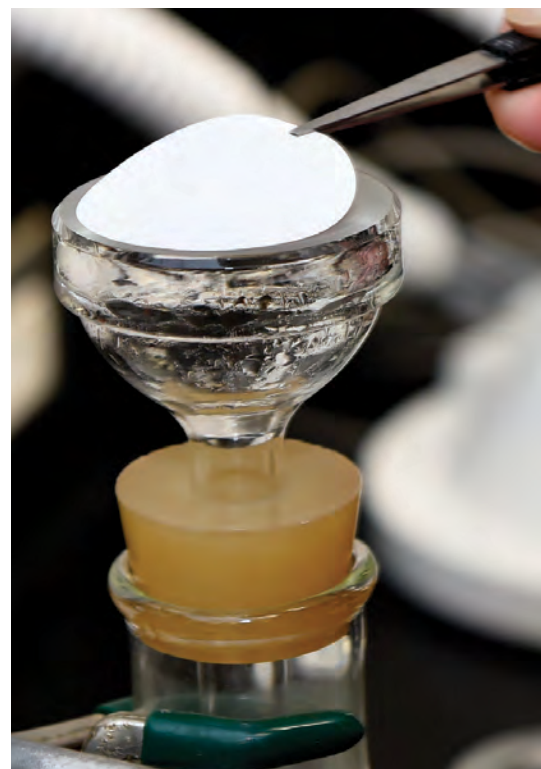
E. coli tests use the standard membrane filter method.
