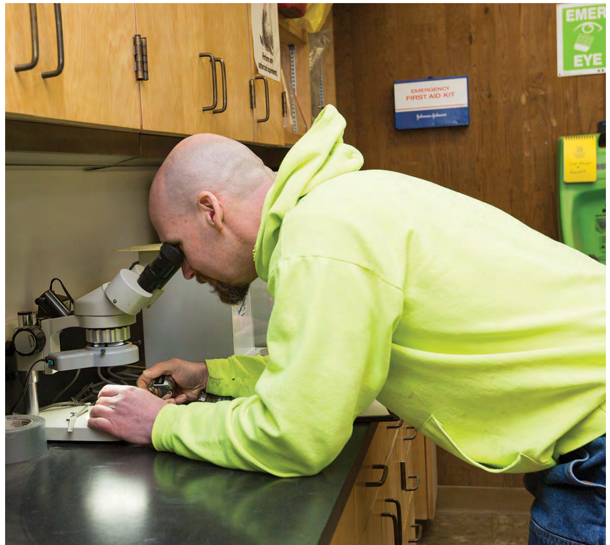
Justin Haley counts fecal coliform colonies. Chlorine dosing in summer helps control fecal coliform in plant effluent, although the plant’s permit does not require chlorination.
