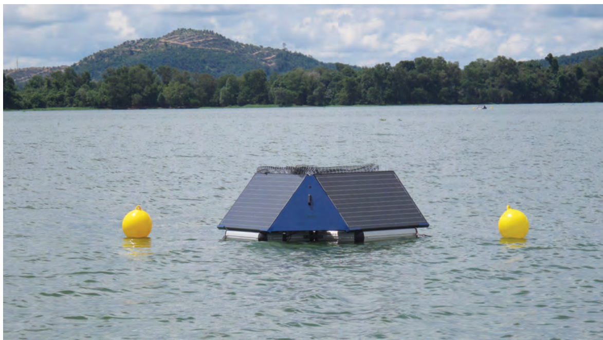
Ultrasonic waves target gas vesicles in the algae, causing them to become less buoyant and sink.
