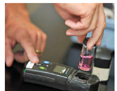
Water samples are tested regularly for chlorine content.
