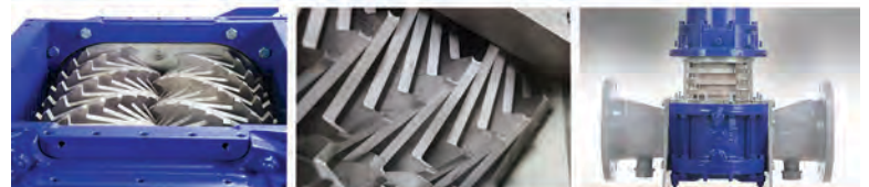
SLUDGE PUMPING SLUDGE GRINDING SLUDGE LYSING
