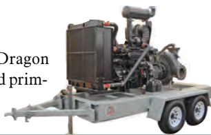
Mobile water-transfer pumps from Dragon Products
