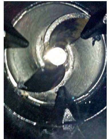
The final impeller design extended the height and length of the vanes to create an auger that doubled as a cutter rotating against the original stationary cutter.
