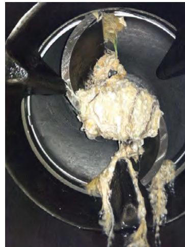
The impeller with S-shaped vanes and recessed lock screw head needed more action to release rags from the smoother profile.
