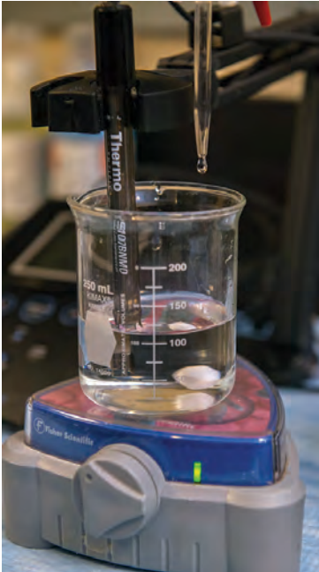
Staff members use a pH meter (Thermo Fisher Scientific) to perform total alkalinity tests.
