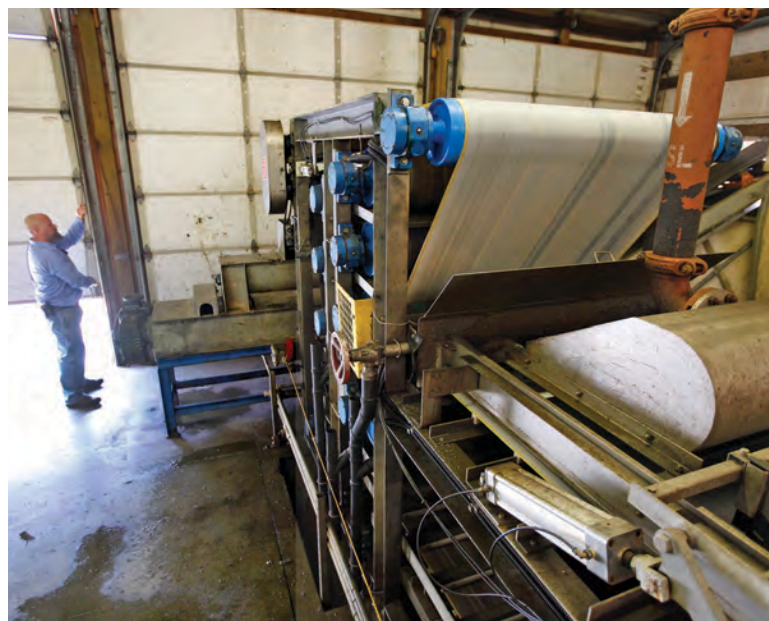
A belt filter press (Charter Machine Company) produces cake that later is mixed with wood chips and yard waste to create compost. Ed Matheson is shown opening a garage door in the building that houses the press.
