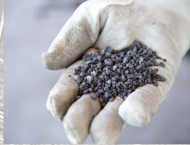
The Tooele facility produces Class A biosolids used as fertilizer on city parks and a golf course. (Photography by Sallie Shatz)
