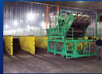
Agitated and Aerated In-vessel type Composting System (ICS)
