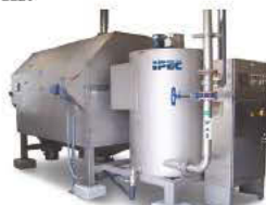
IFT rotary drum sludge thickeners from IPEC Consultants
