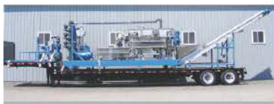
Belt filter press system from Bright Technologies
