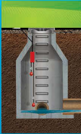
In Sewer Level Alarm
