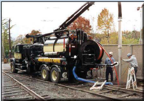
SEWER & CATCH BASIN CLEANING Single and double-pump jet-vac combination units with line jetting capabilities of 175 gpm. Catch basin cleaning available with per hour or per basin pricing.
