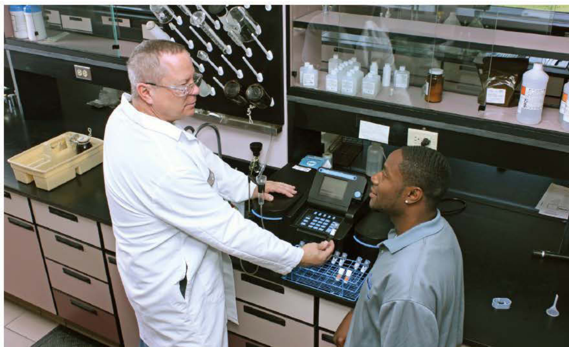
Tillis and lab technician Joe Valerius test phosphorus and chlorine levels in the Beloit treatment plant microbiology laboratory (Hach DR/4000 U spectrophotometer).
