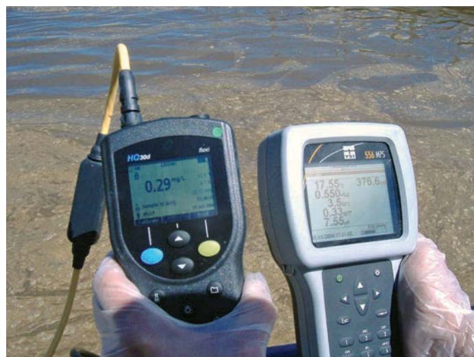
Dissolved oxygen readings are shown on a Hach LDO meter and a YSI 556 multimeter.
