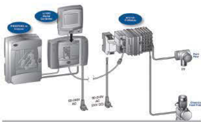
RTC 101 phosphorus control system from Hach Co.
