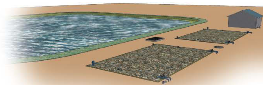
The Mentone Wastewater Treatment Plant uses two Submerged Attached Growth Reactor (SAGR) beds for post-secondary treatment.
