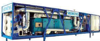
Advanced anaerobic digestion system from Siemens Water Technologies
