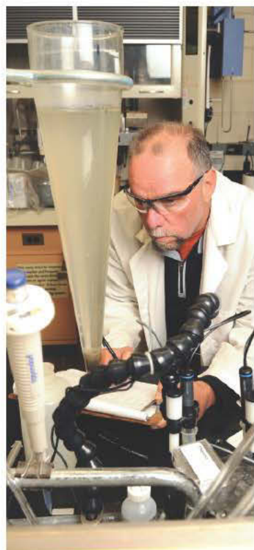
John Riccio uses an Imhoff cone to perform a test to measure settled solids.
