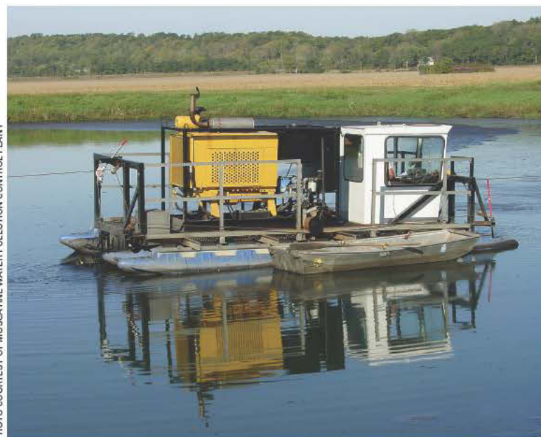
Crews use a dredge to draw biosolids from the lagoons for land application.
