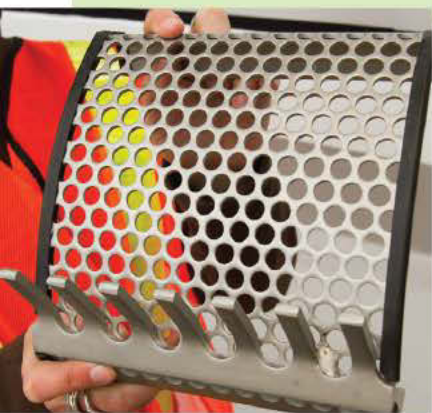
Sample section of the 9 mm punch plate screen design (WasteTech, a Division of Kusters Water) in the plant headworks.
