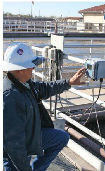
Jodey Lane checks an LDO probe from Hach.
