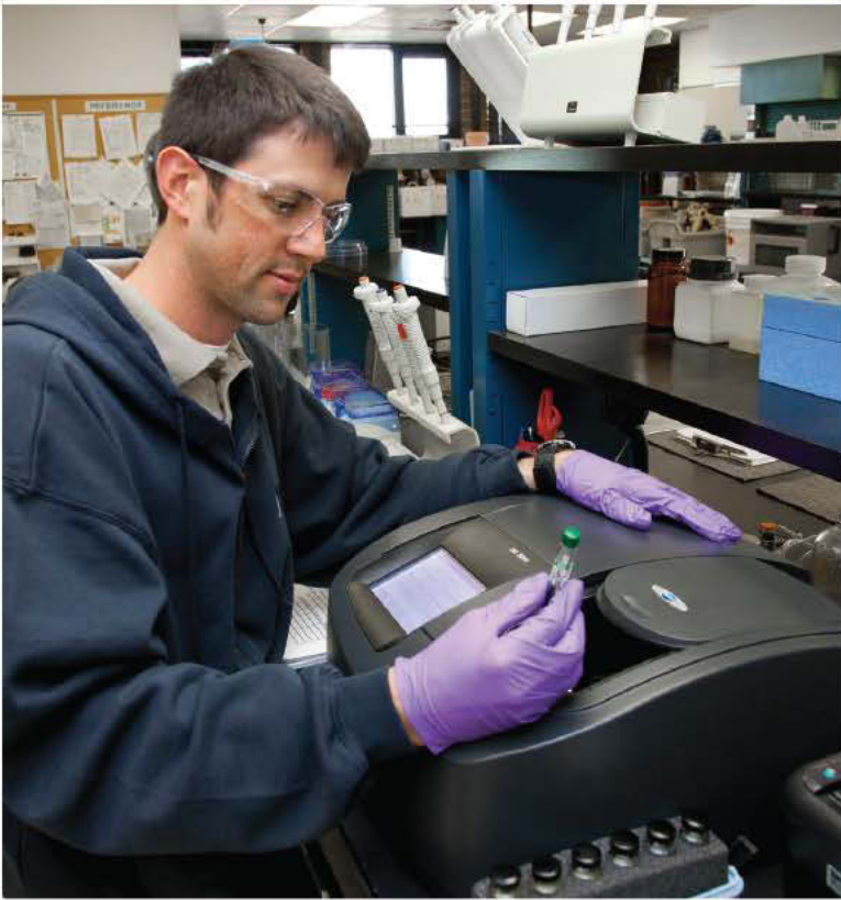
ABOVE: Laboratory technician II Kevin Hardee tests samples (Hach DR 5000 spectrophotometer). BELOW: Wastewater treatment plant operator III Warren Harris checks a control panel (Tetra Tech).
