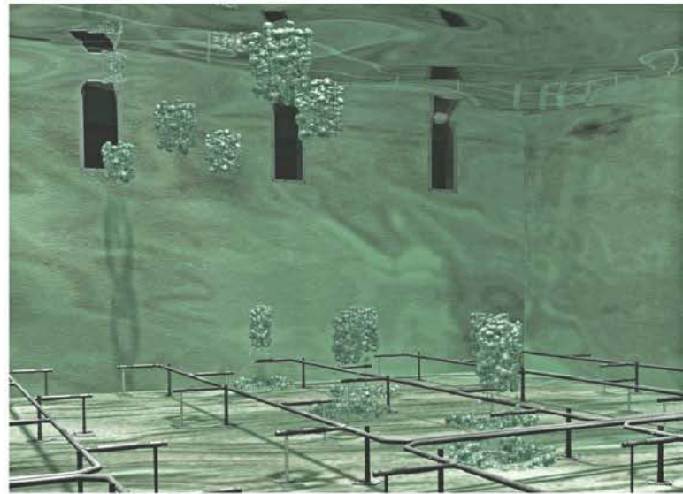
FIGURE 1 – The large-bubble system uses compressed gas (air, nitrogen, methane) to intermittently and sequentially fire programmed short bursts of softball-sized bubbles from engineered, floor-mounted nozzles.
