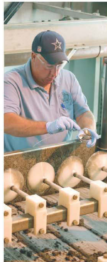
Operator I Steven Belote collects samples at the biosolids belt press (Komline-Sanderson).
