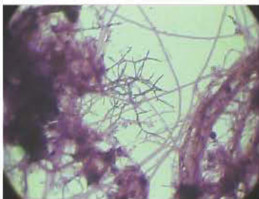
FIGURE 2 – Nocardia was identified as the culprit causing the foam. Nocardia is one of several fungi that cause foaming in activated sludge facilities. It is relatively easy to identify, since it is a short, truly branched filament that is gram positive and mostly Neisser negative.
