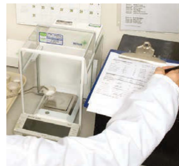
A METTLER TOLEDO balance is used to weigh crucibles for TSS testing.
