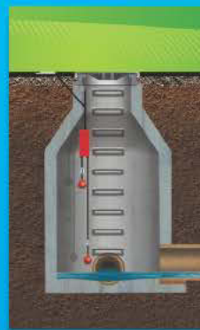
In Sewer Level Alarm
