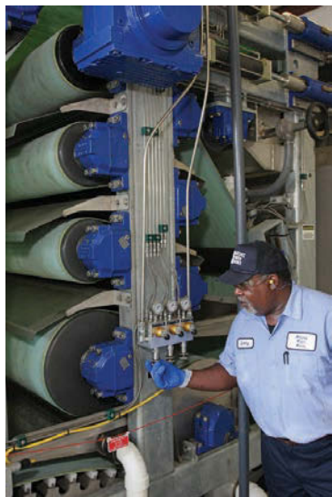
Operator Larry Young adjusts belt tension on the BDP Industries belt press.
