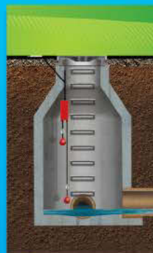
In Sewer Level Alarm
