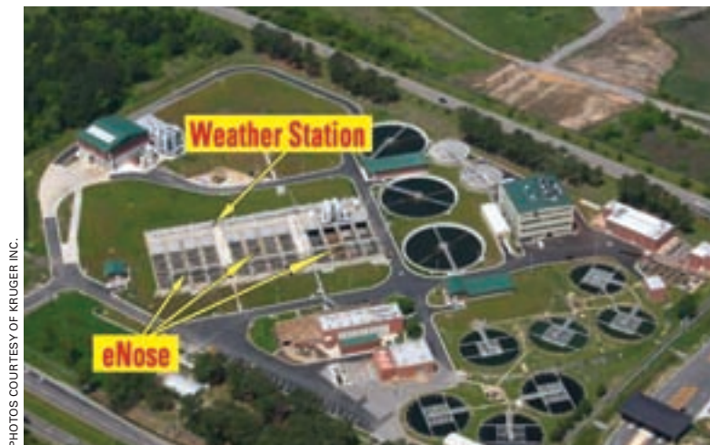
Locations of the weather station and eNoses that are parts of the OdoWatch monitoring system are shown on an aerial photo of the Hampton Roads Sanitation District treatment plant.
