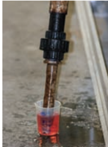
ABOVE: Operator Randy Oesch operates the Ashbrook Klampress belt press. RIGHT: Samples are taken at the aeration basin to measure the ORP/pH balance.
