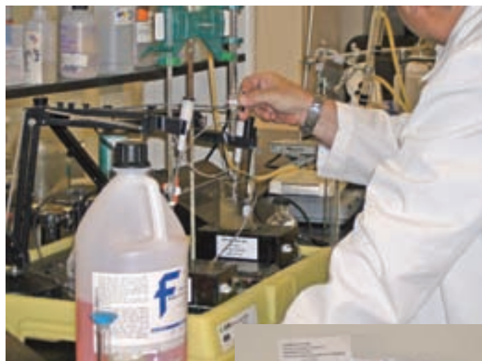
Tests for alkalinity can be performed in the laboratory (above) or in the field using simple and inexpensive test kits (right).
