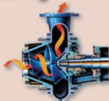
WEMCO-HIDROSTAL Screw Centrifugal Pumps
