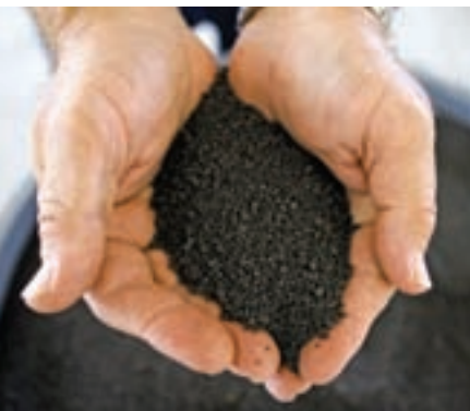
The plant produces Class AA bio-solids pellets in a natural-gas-fired Andritz dryer that heats up to 1,200 degrees F.
