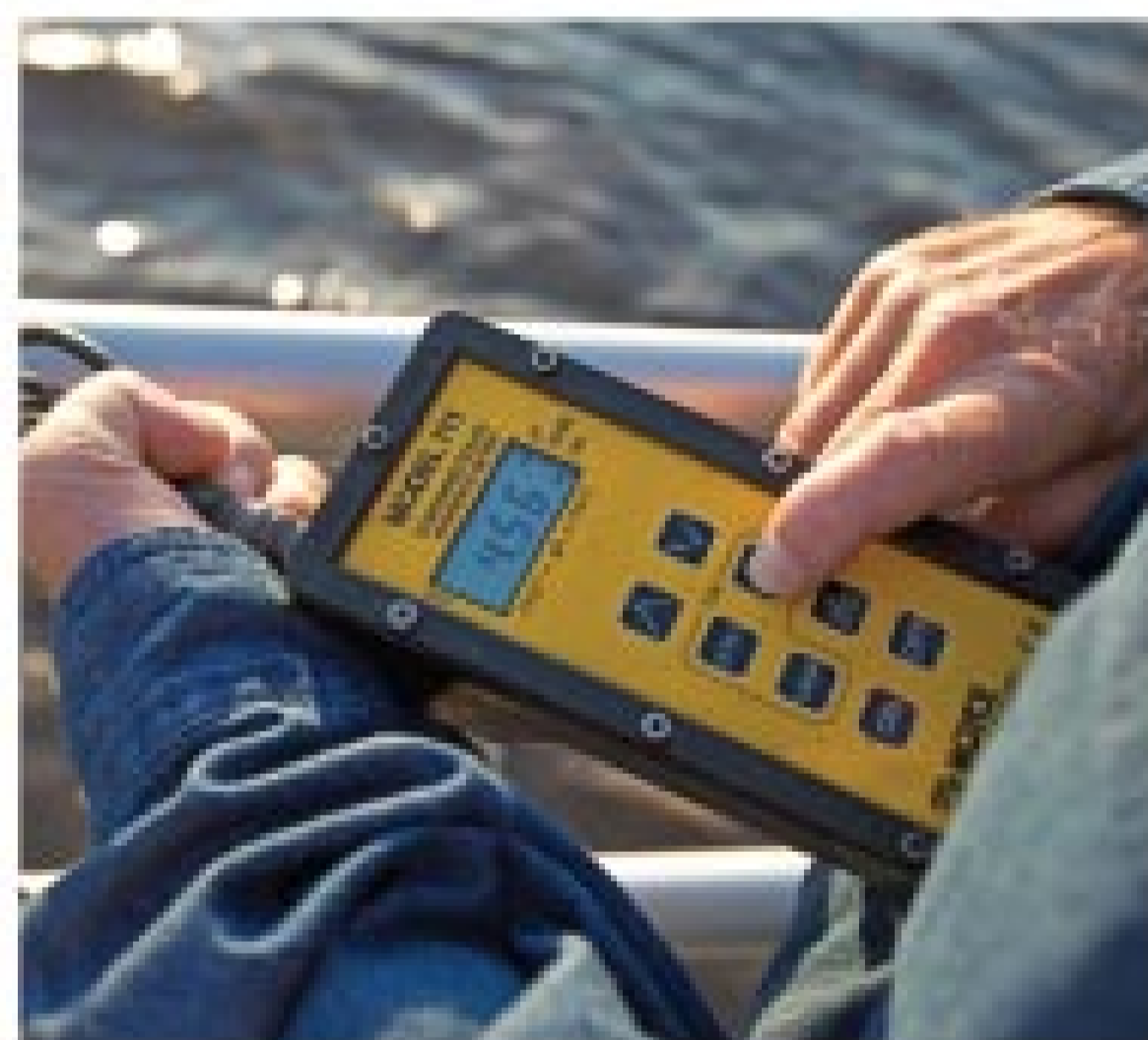
ABOVE: Class 4 operator Pat Fountain takes one of the daily water samples used to check for E. coli and other bacteria, as well as ammonia. LEFT: A Royce handheld TSS meter is used to test for mixed liquor suspended solids in the aeration basin.
