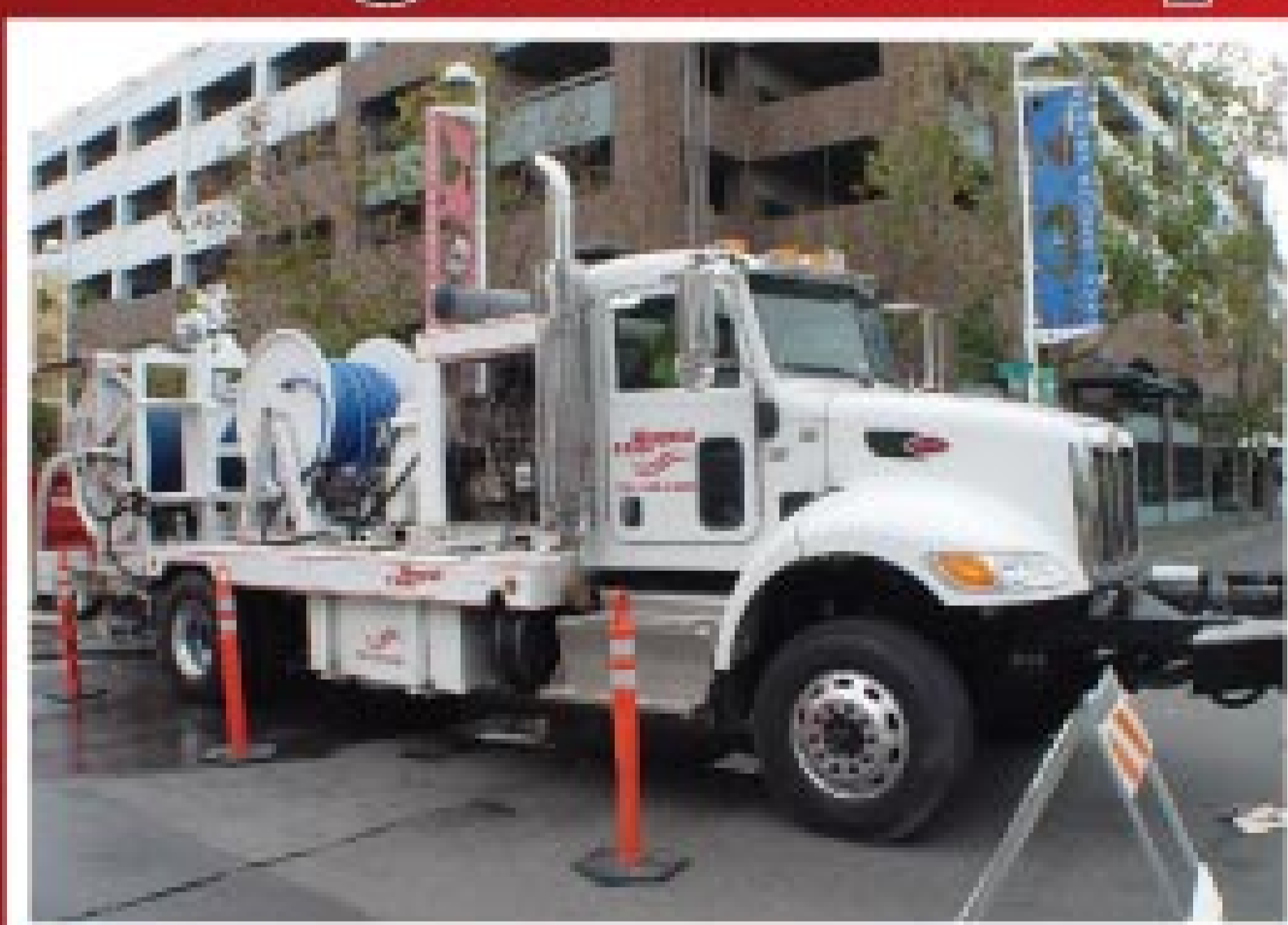
JT180 Jet Truck Produces 360 GPM @ 2000 PSI
