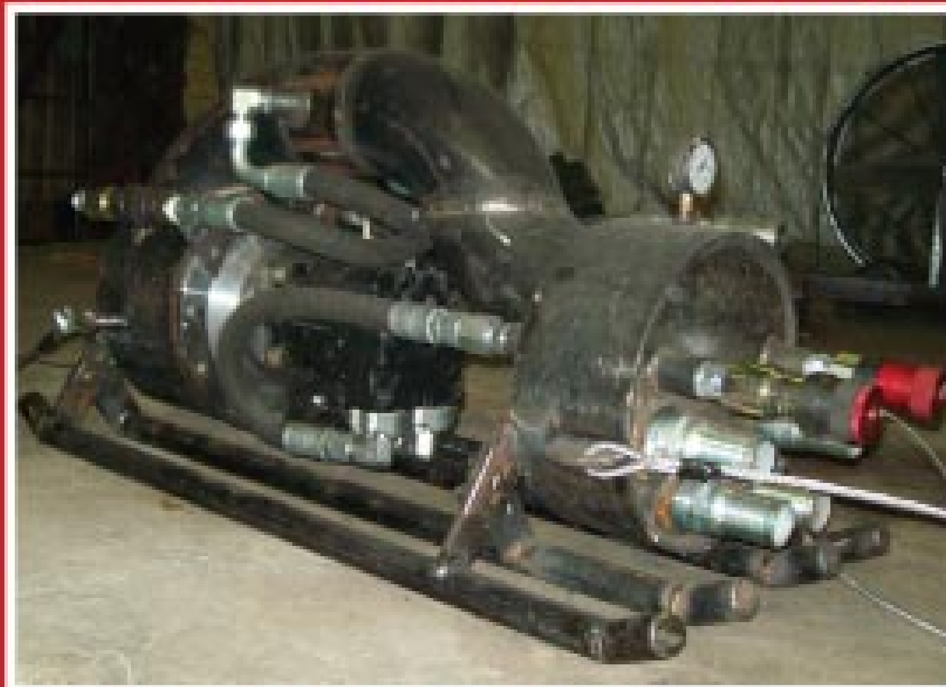
2000 GPM Tsunami Nozzle Uses Sewer Water
