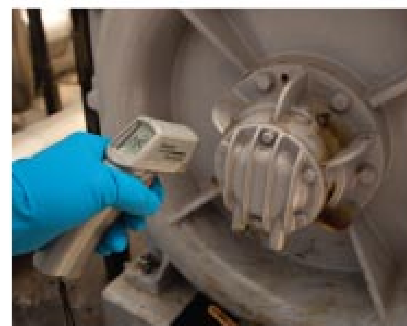
A mechanic checks the temperature of a repaired bearing using a Raytek handheld thermometer.
