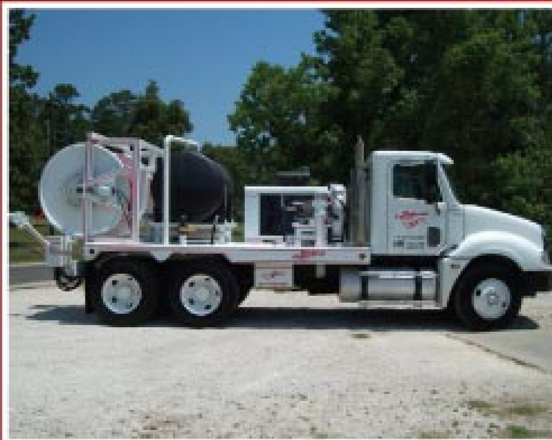
JT180 Jet Truck Produces 360 GPM @ 2000 PSI
