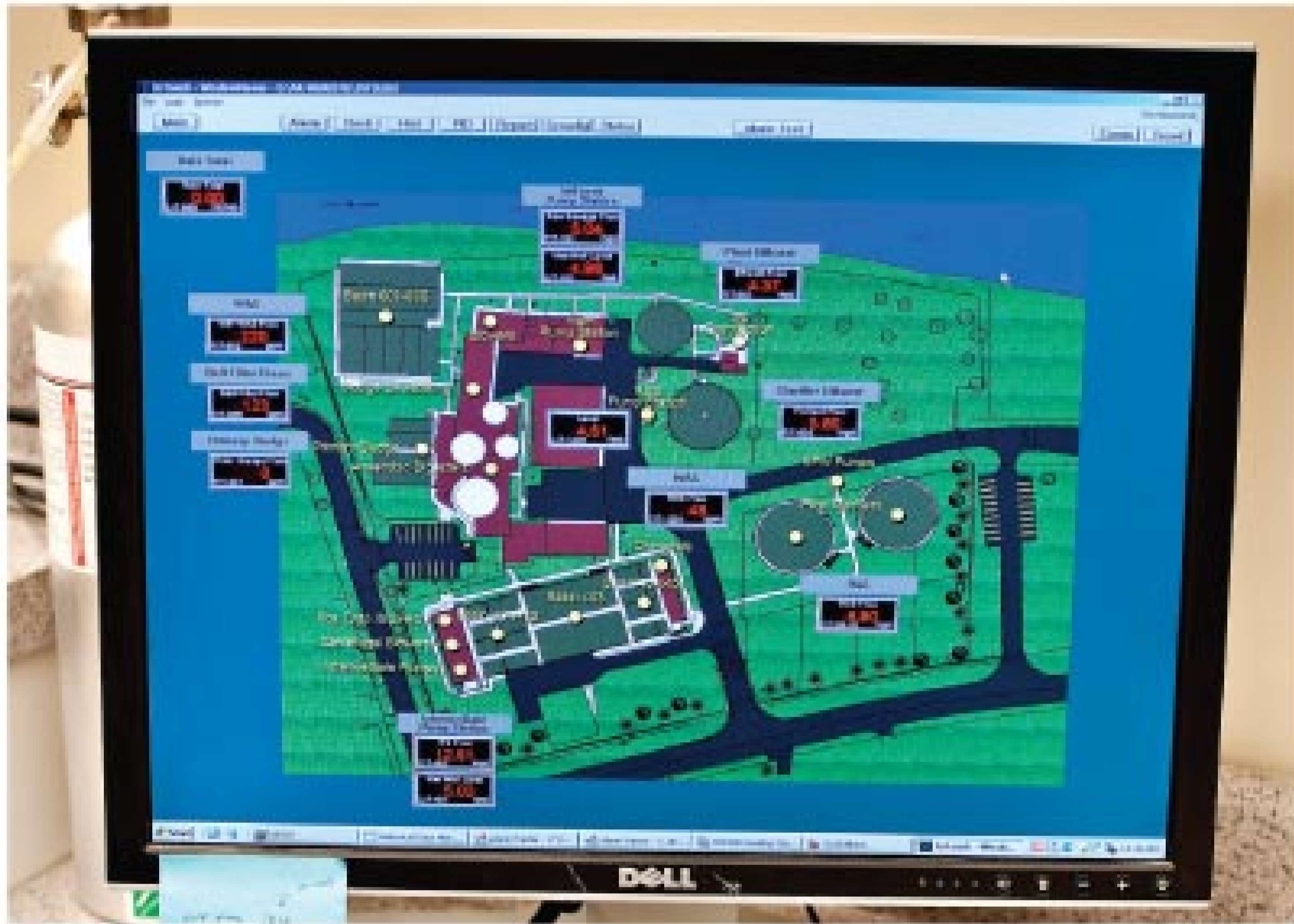
ABOVE: One of the two final Envirex Tow-Bro circular clarifiers. BELOW: The plant's SCADA system, which includes PLCs from Allen-Bradley (a division of Rockwell Automation) and Intellution software. The system provides monitoring and control at five locations within the plant as well as on staff laptops.
