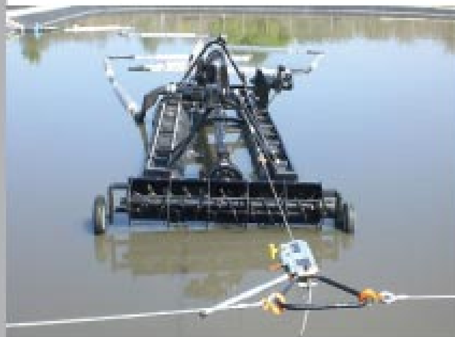
Flump dredge from SRS Crisafulli Inc.
