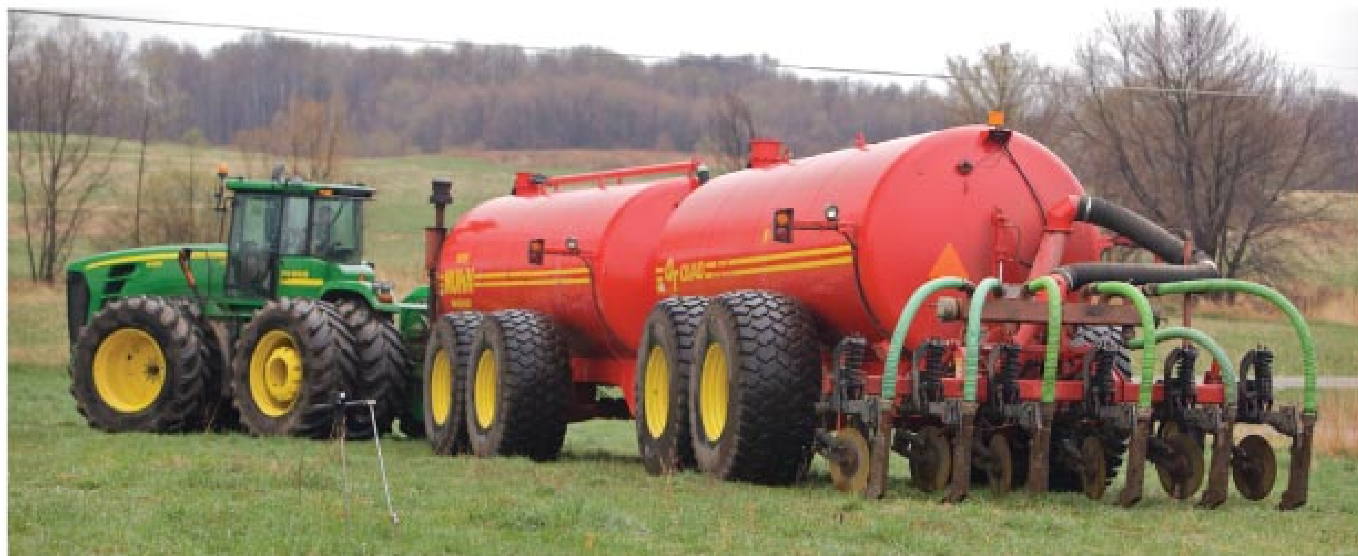
Biosolids are land-applied with a John Deere tractor pulling a Nuhn Quad Train applicator from Nuhn Industries Ltd. Farmers report excellent results from biosolids applications.
