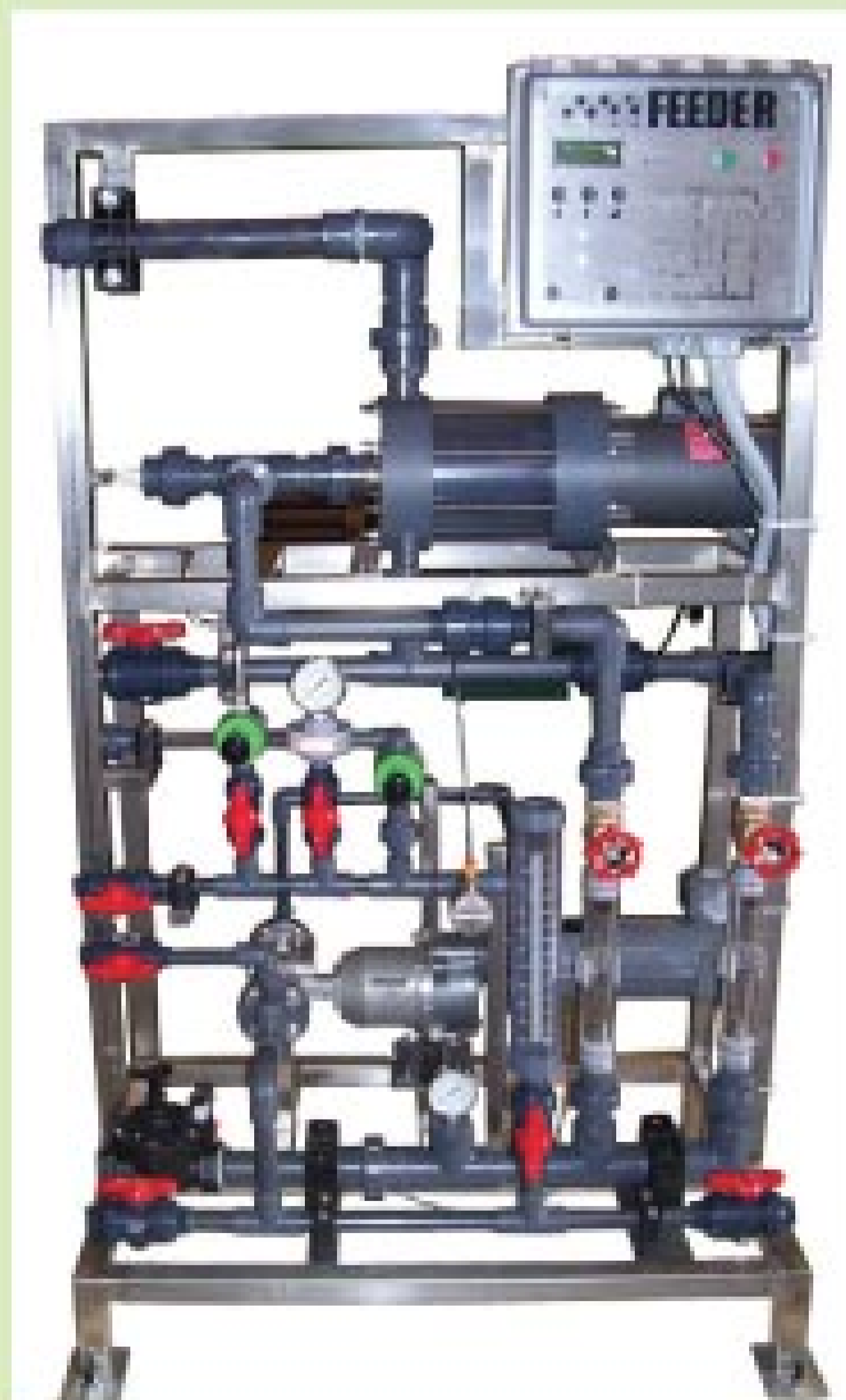
Polyfeeder emulsion polymer blending system from Pulsafeeder Inc.
