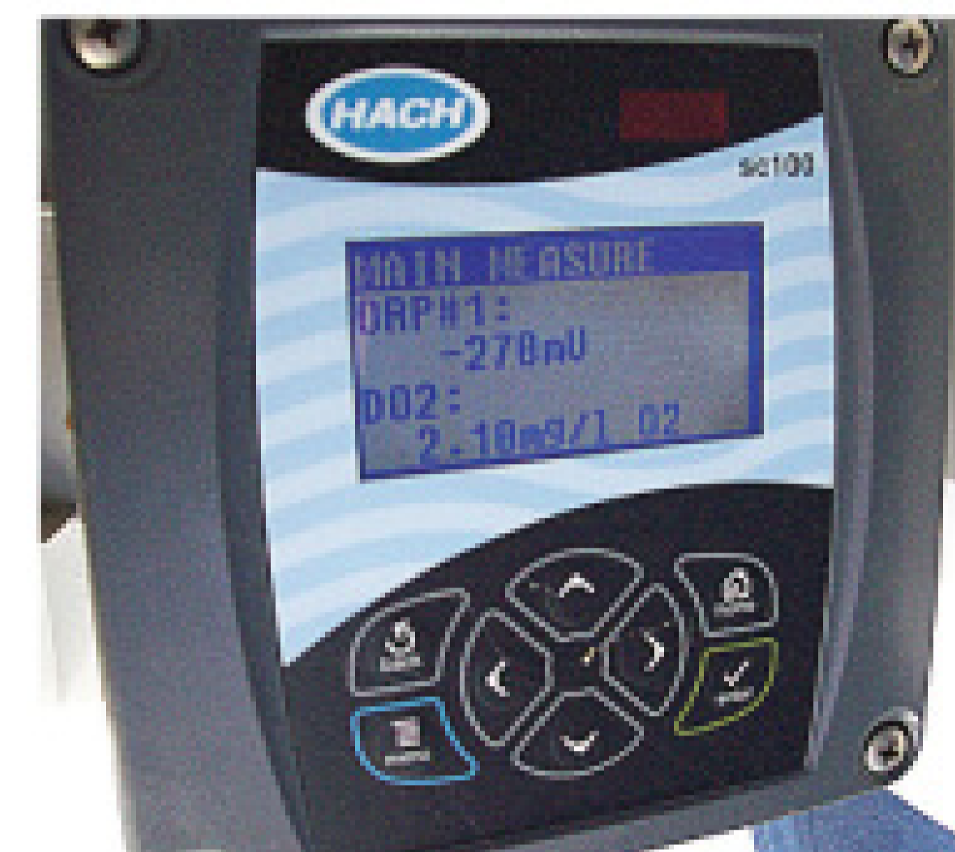
ABOVE: American-Bath chief operator Jeff Bassitt downloads data from the Hach sc100 controller. With inline meters providing real-time and historical DO and ORP values, Bassitt and colleagues can establish trends to optimize DO control and determine the time and cause of transient conditions. RIGHT: The probes plug into Hach sc100 controllers that continuously read the process sensors and can communicate via a 4-20 mA signal to a plant's PLC or SCADA system.
