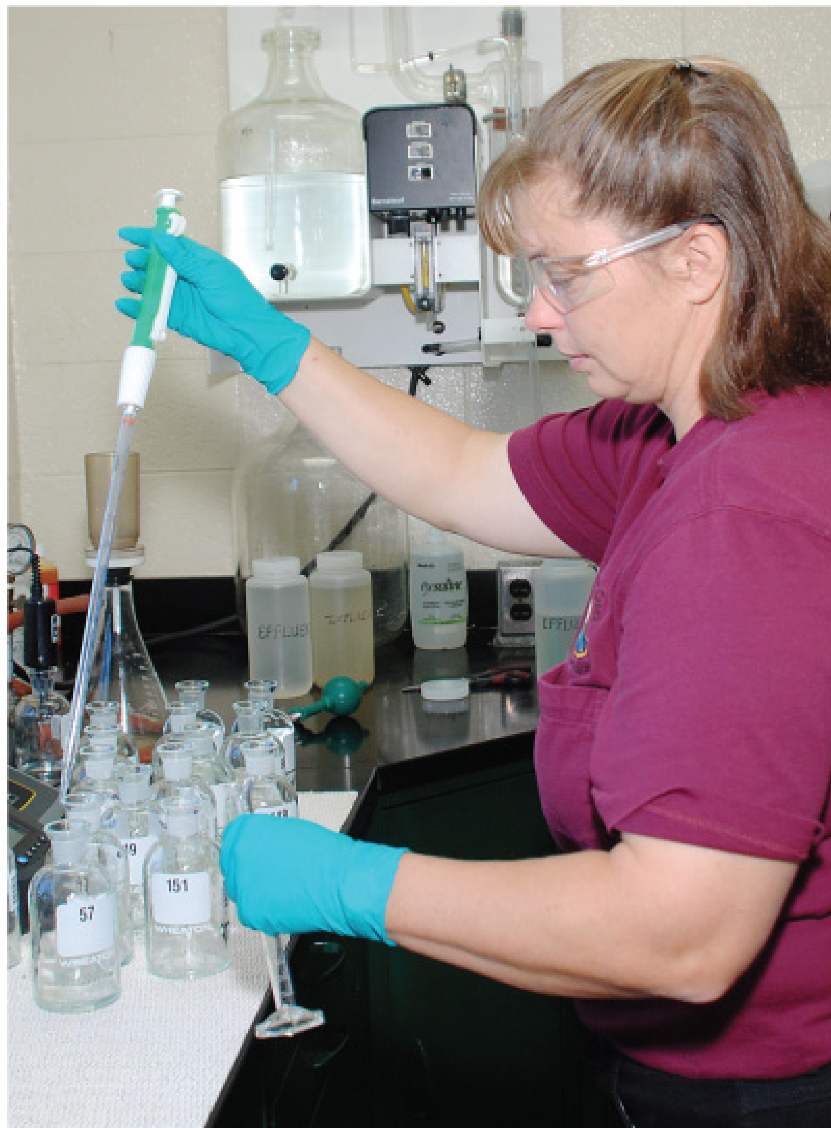
Annetta Grillo sets up BOD samples for testing.
