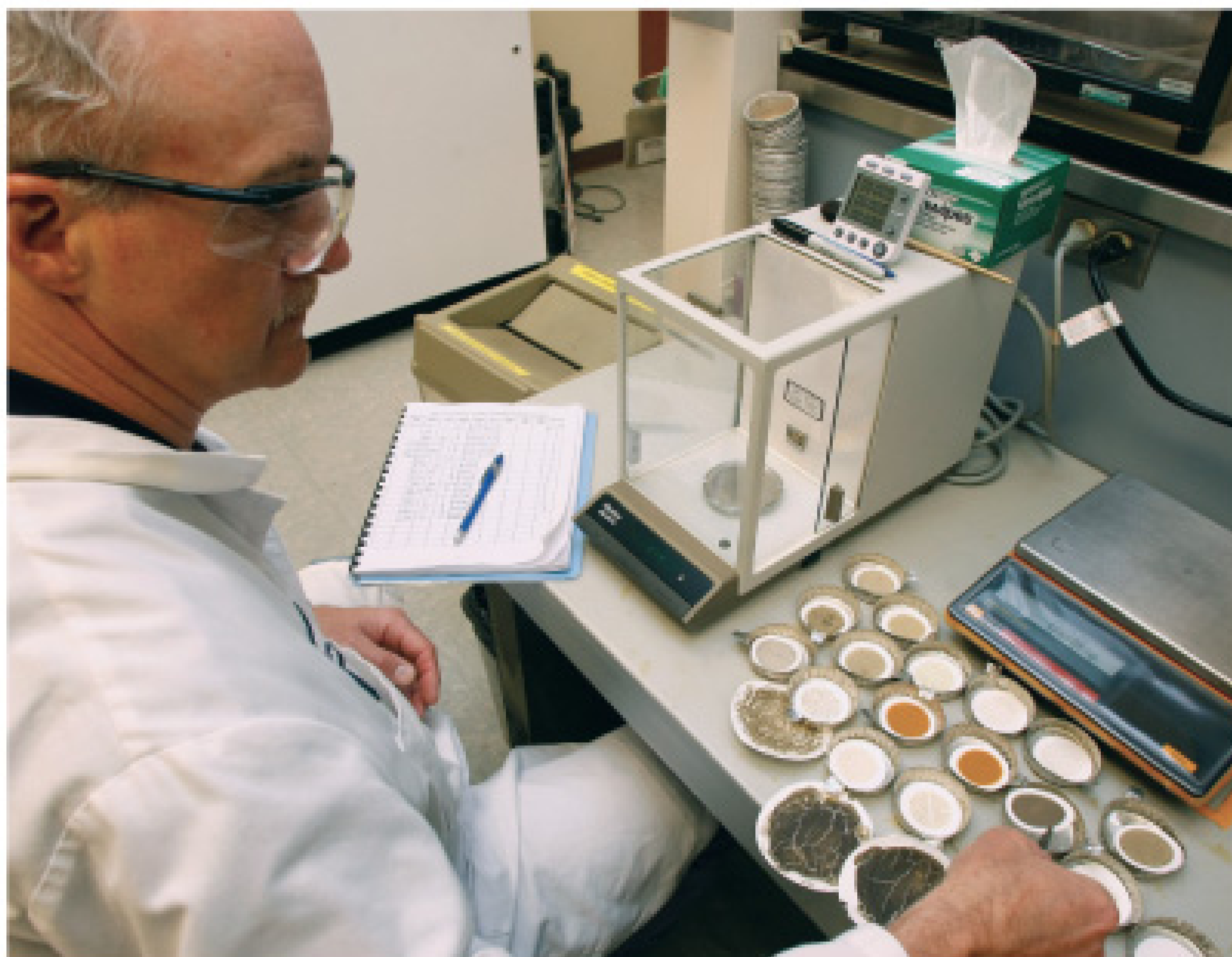
LEFT PHOTO: Water quality analyst Tim Rickman weighs wastewater solids collected on clarifier filters to determine TSS at different stages of clarification. ABOVE: The view east from the primary clarifier shows the secondary clarifiers, in the foreground, and two trickling filters.
