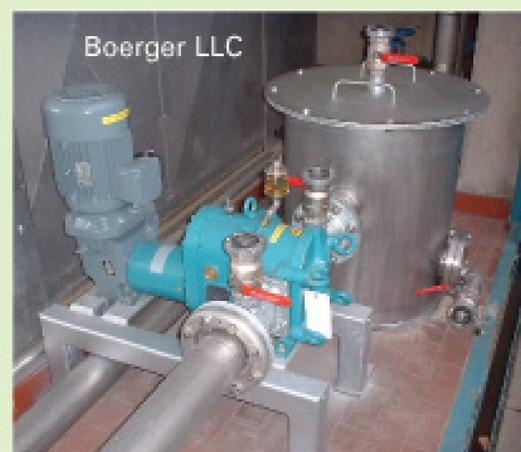
catchers and control panels. When used in tandem with the company's rotary lobe pump technology, benefits include identical quenched mechanical seals and other components that allow consolidated parts inventories. With Maintenance In Place (MIP) features, inspection and maintenance can be performed without disconnecting piping or drives. **877/726-3743; www.boerger-pumps.com.**
