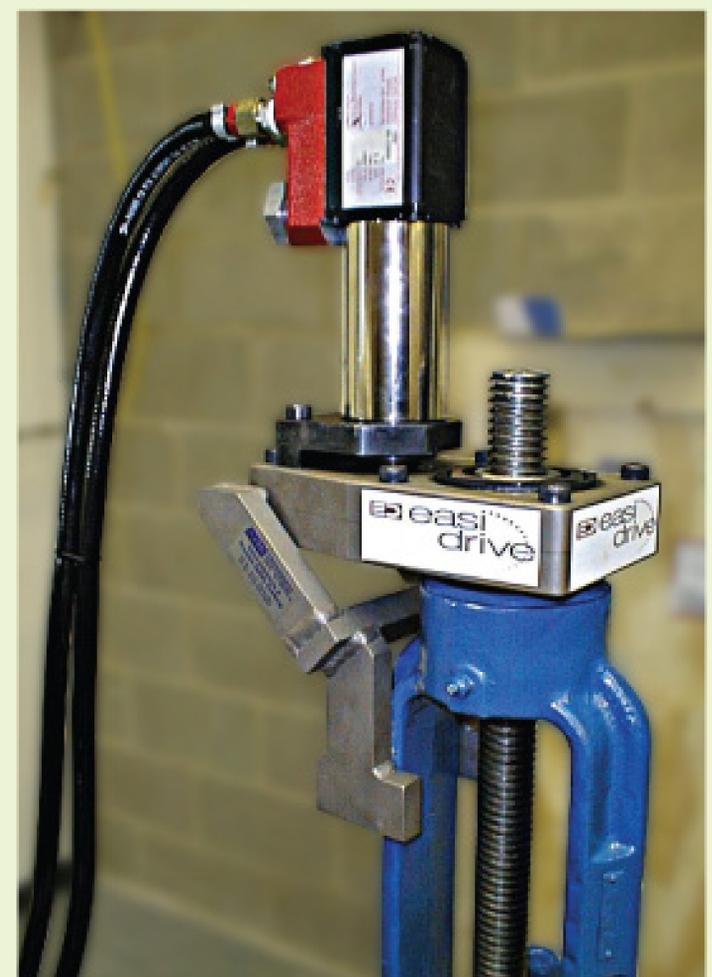
Easi-Drive portable valve operator from Smith Flow Control Inc.
