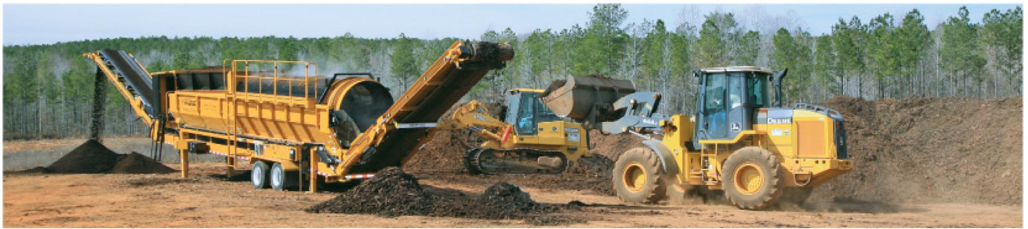
After the 180-day windrow period at the compost facility, a Wildcat trommel screen is used to separate the finished product from any larger debris. The debris is moved back to the open-air shelter where it can be reused.
