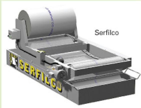
Filtered solution can then gravity drain to waste or be returned to the process by a pump. Consumed fabric is advanced to the sludge box as fresh media and simultaneously indexed to the solution flow. The unit is available in carbon steel, 316 stainless steel, CPVC or polypropylene, in sizes from 1.5 to 113 square feet of filter surface area and flow rates to 650 gpm at 80 micron. **800/323-5431; [www.serfilco.com](http://www.serfilco.com).**
