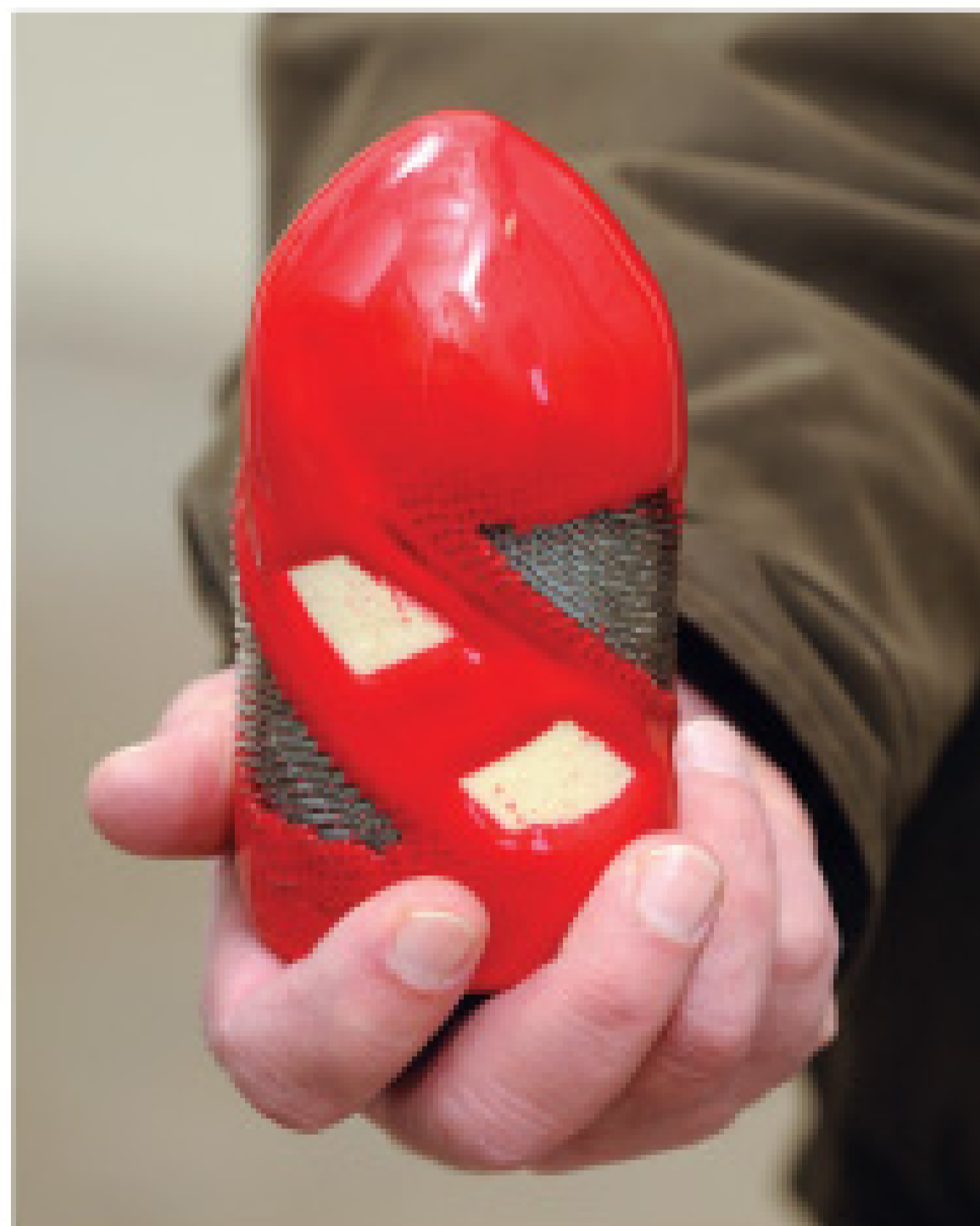
ABOVE: Jordan Kleinsmith takes readings from gauges that monitor the BioPasteur process heat exchanger. LEFT: A pig from Pipeline Pigging Products is used to scour heat exchanger lines. RIGHT: The BioPasteur system uses three 3,300-gallon tanks that operate in a sequential batch mode.
