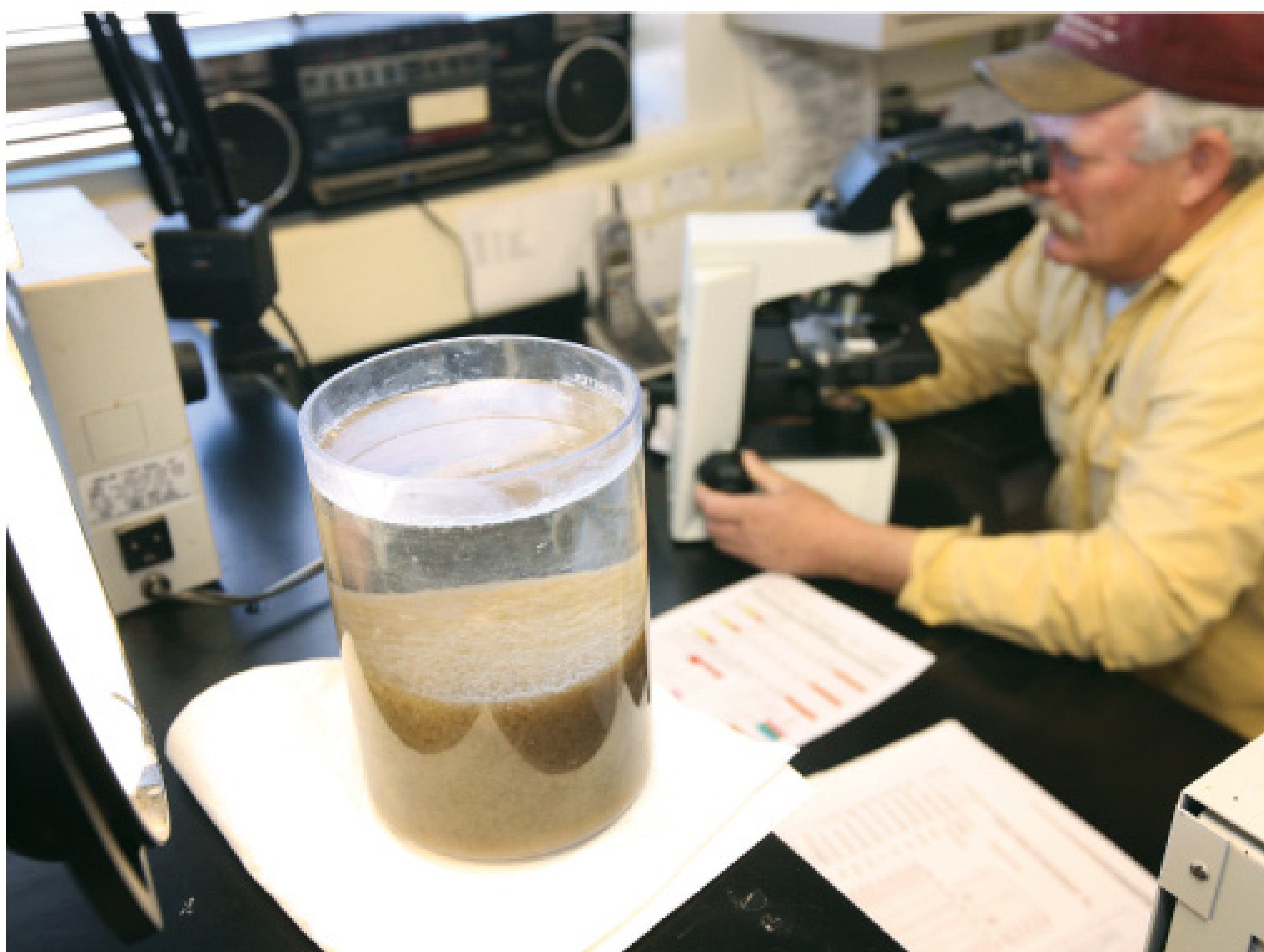
Glen Anderson examines the organisms in a return activated sludge sample. He can confirm the health and relative age of the solids in the plant using this method. (Photography by Jonas Grushkin)
