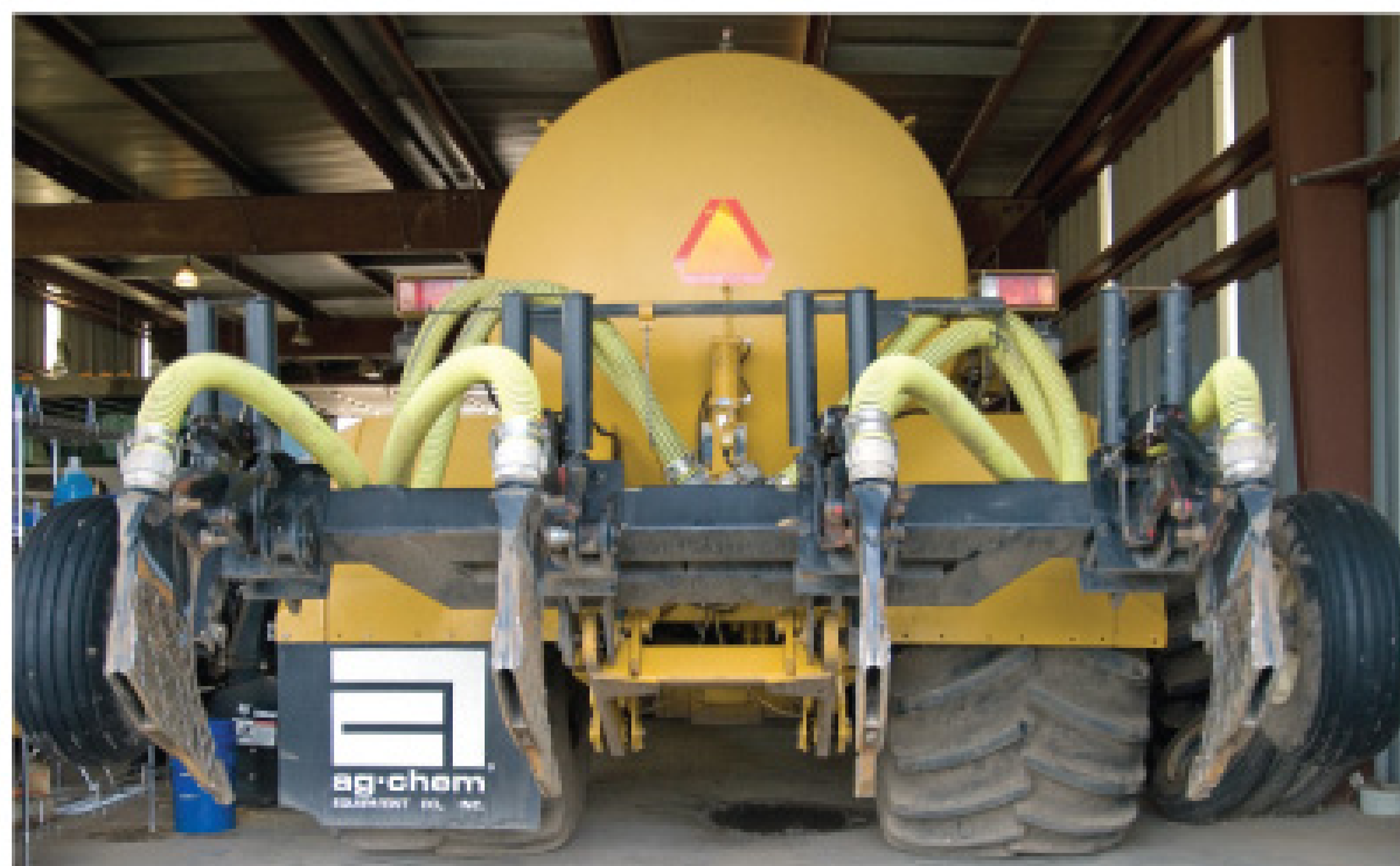
A TerraGator vehicle from AGCO Corp. injects biosolids into cropland. The four tines till the soil
