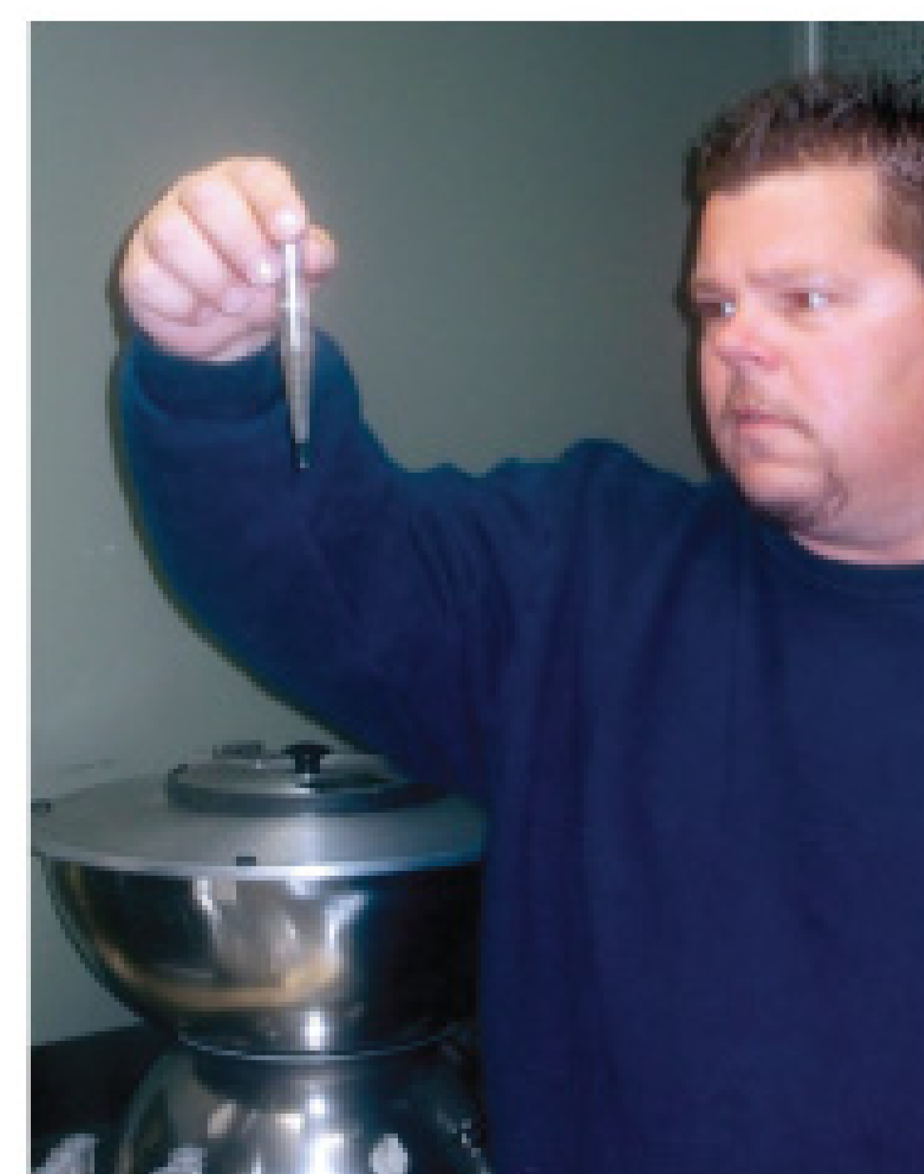
Guelph treatment plant team member Mike Innocente checks the amount of sludge that has settled after a centrifuge spin test.
